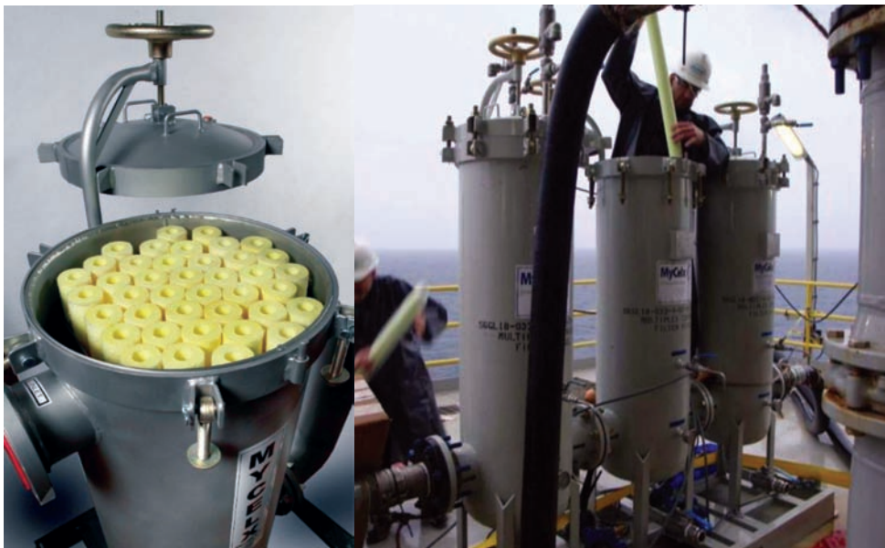
MyCelx filters within single vessel of the MyCelx Polisher and MyCelx Polisher being loaded with MyCelx filters on site
