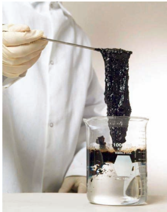
Laboratory Demonstration of Oil Cohesion resulting from use of MyCelx polymer
