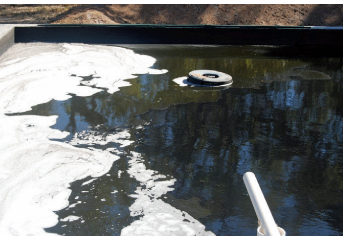
▲ Water at fire-training site showing foam, phase separated oil and oily emulsion in 30 KL retention tank. 📷 OLEOLOGY
