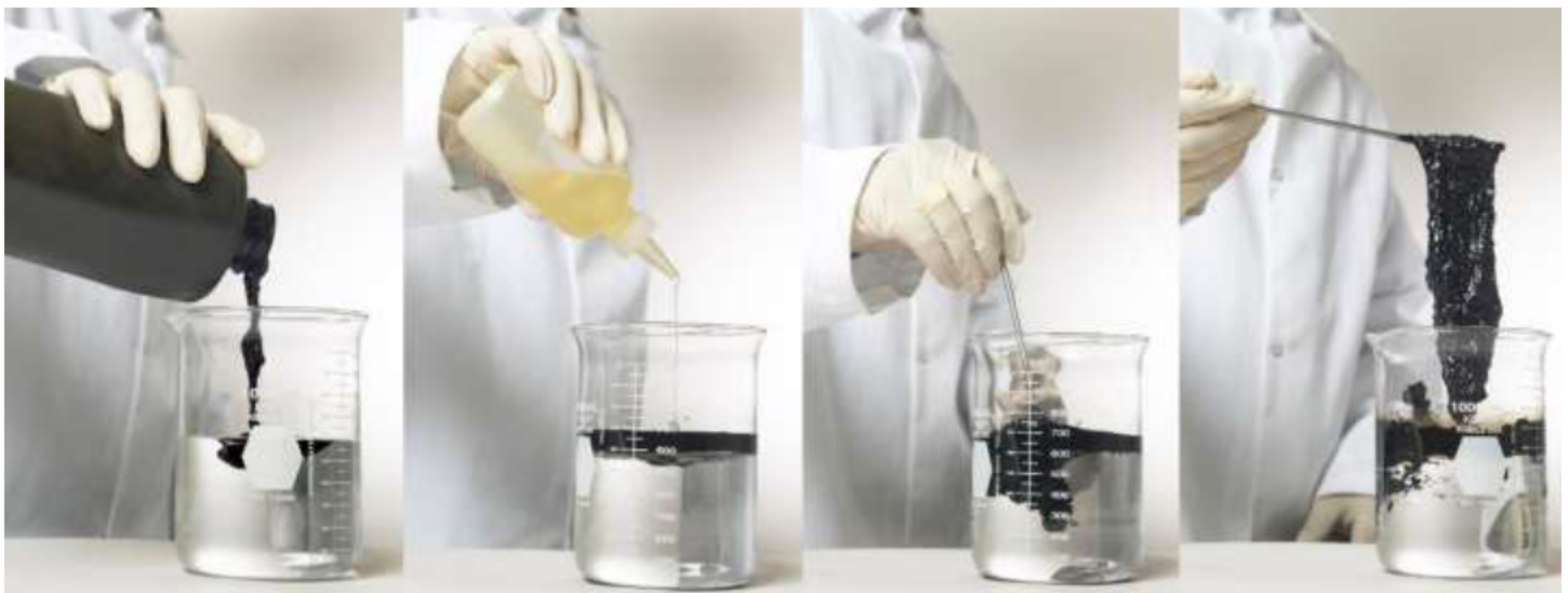
Above: Crude oil added to a beaker, MYCELX liquid polymer chemistry added, once the polymer comes in contact with the oil, it forms a cohesive singular mass.
