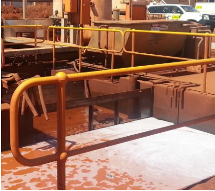
The mine site collection sump with evident detergent clearly visible & Filter system as installed
