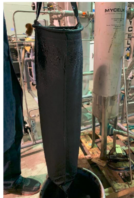
Photo of MYCELX Extended Life Bag Filter being removed after use during testing. Many of these filters were tested and the average oil holding capacity was determined to be 8.8 lbs. oil
