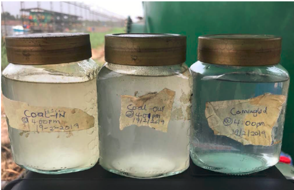
TYPICAL WATER QUALITY INTO SYSTEM, FROM LEFT TO RIGHT, INLET, OUTLET OF COALESCER, OUTLET OF REGEN (NO POLISHER IN USE)
